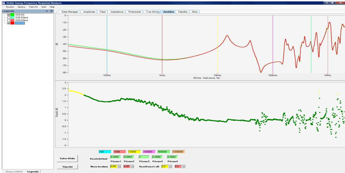
Fig. 3: Analysis of waveforms D25-D0 (reference and from type tests) for open circuit measurement methodology using cross-correlation coefficient
