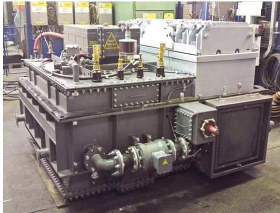
Fig. 2: Railway traction transformer prototype. Type T1T-4900-25/2x1700 [2]
