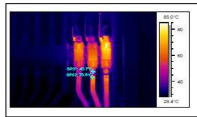
Fig.5: Thermogram of electric wiring breaker
