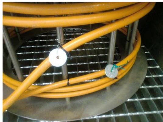
Fig. 8: Cables after simulated 40-year operation in the primary circuit (with no visible damage and change in the sheath colour)
