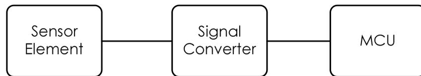
Fig. 1: Block diagram of a basic sensor unit
