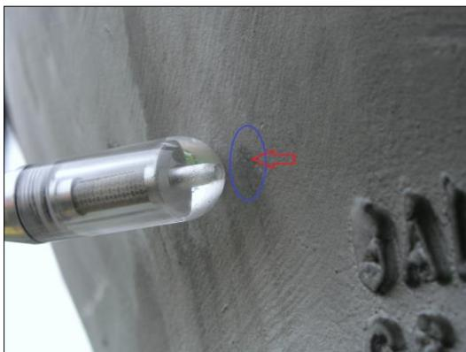
Fig. 5. Place of leakage – probe of sniffer
