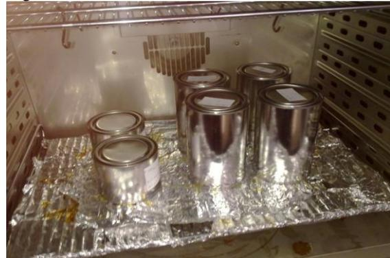
After 168 of influence 40°C water on samples we took them from water dry them with filter- paper and measured their insulation resistance immediately after test and after one and two hours after test in water. Results are in Tab.5
