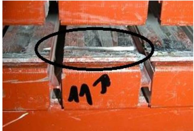
Fig. 7. Defect made by a touch of grinding machine at the side of the tooth.
