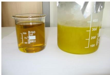
Fig. 1. The difference in the appearance of Fatty Acid Methyl Ester at different temperatures (at left at 20 °C, at right at -20 °C)
