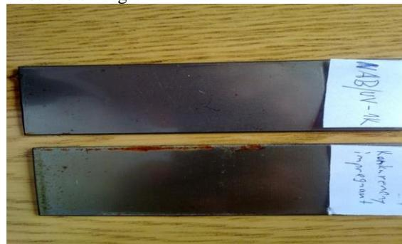
From results of volume resistivity, moisture absorption and rust resistance is our resin better as competitive resin. Our resin has 3500 times higher volume resistivity after influence of water as competitive resin. Absorption of moisture is about 35% lower as has competitive resin. Rusting of Fe plates is lower as has competitive resin.
