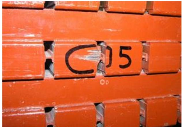
Fig. 3. Defect made by the chisel.
