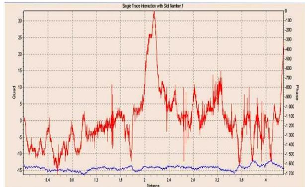
Fig. 2. EL CID record – no faults.
