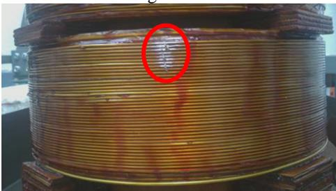
Fig. 6. The created interturn axial short circuit on the phase A
