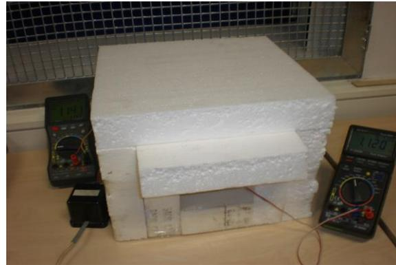
Fig. 1. Arrangement for thermal conductivity measurement.
