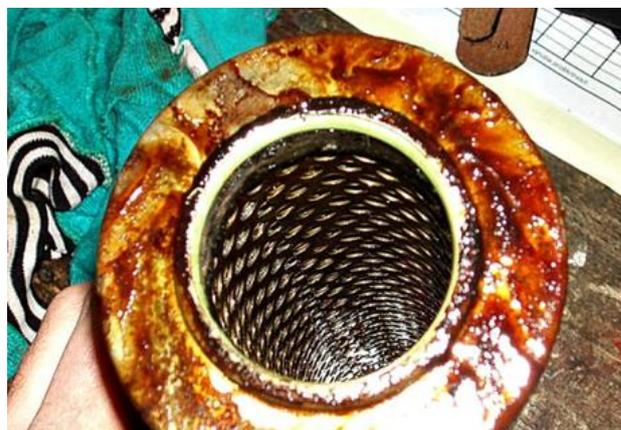
**Fig. 1** Oil filter covered by resin-like material of oxidation products
