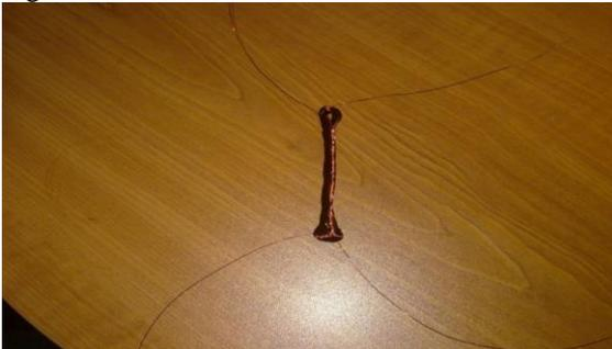
For comparison we wound twisted coils from wire STN EN 60317-13 Gr.2 with diameter 0,71. We wound 15 coils, because diameter was bigger. These samples are in table 4 designed G2.
