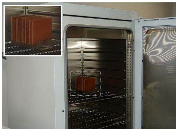
Fig. 1. Test specimens placement in furnace Venticell
