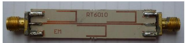
Fig. 2. Fabricated microstrip filter with soldered connectors (RT/duroid6010LM).
