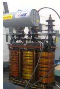
Fig. 1. The tested transformer pulled up from the transformer tank
