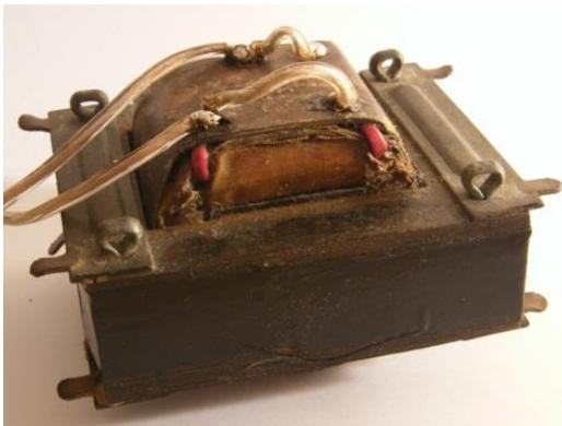
Fig. 4. Measured transformer TESLA 230V~24V
