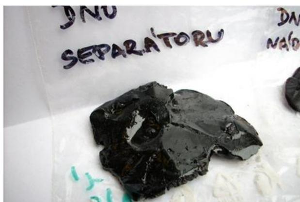
**Fig. 2** Piece of black insoluble material formed by oil oxidation
