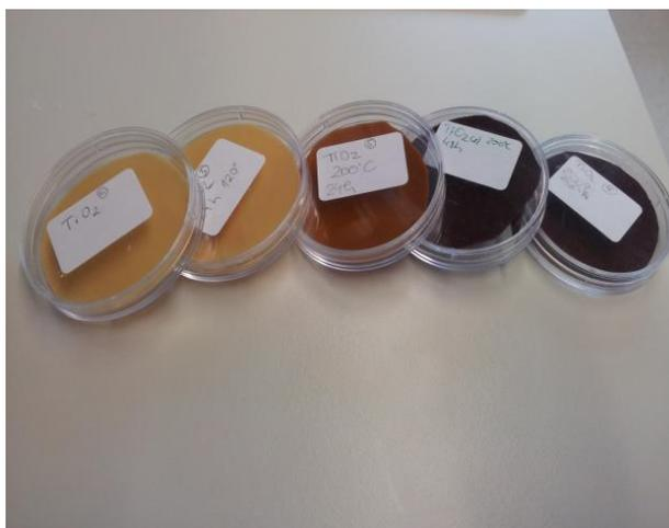
Fig. 4. Final nanocomposites samples at different stages of accelerated ageing
