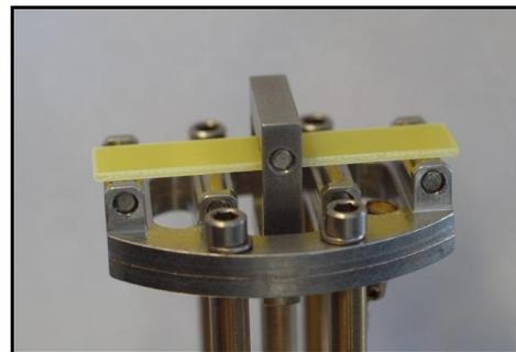
Fig. 4. Placement of the sample in clamps during measuring by DMA method – 3 point bending mode of measurement
