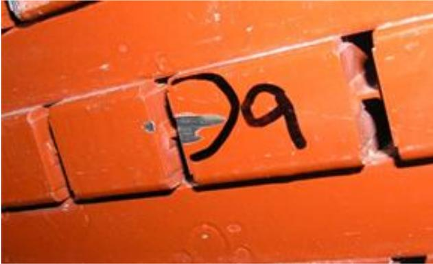
Fig. 4. Defect made by a gentle touch of the grinding machine.
