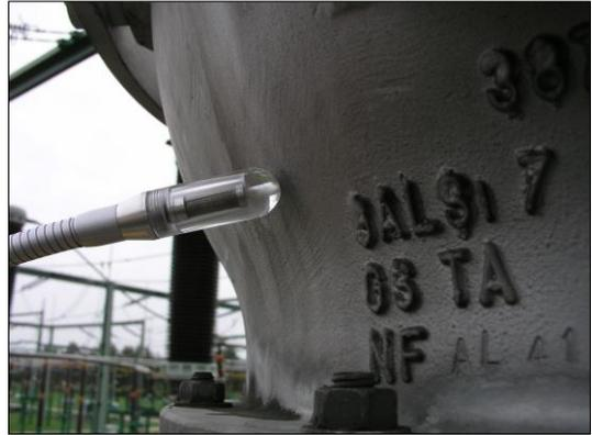
Fig. 6. Place of leakage (above flange)
