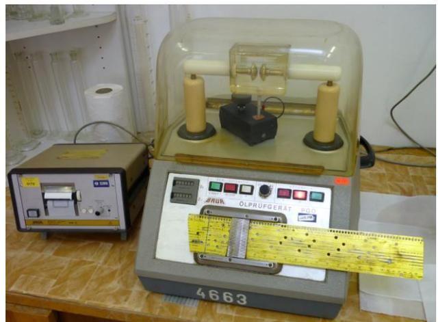
Fig. 3. Measurement of the breakdown voltage – Baur PGO 90 A-2
